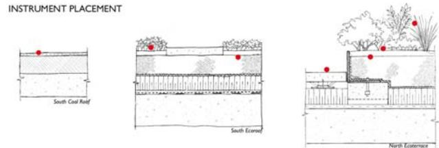
**Fig. 6:** Seven data locations chosen for testing
